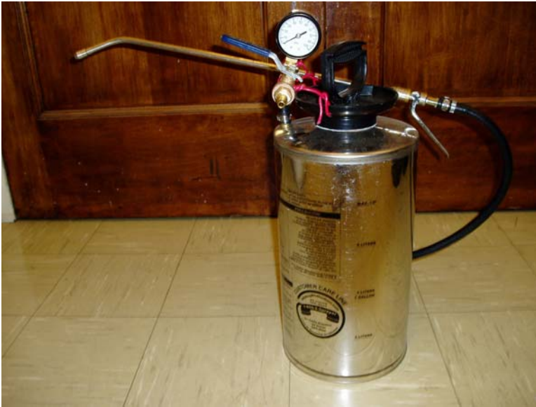
Figure 8. Retrofitted garden sprayer
